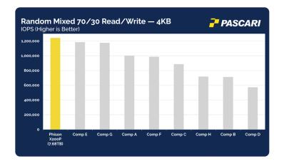
The Pascari X200P delivers the best performance in the demanding mixed random 70/30 read/write testing, beating the nearest competing drives by 5%, and offering up to double the performance compared to other enterprise SSDs. That's thanks to the high-performance controller and NAND, coupled with Phison's firmware expertise.
